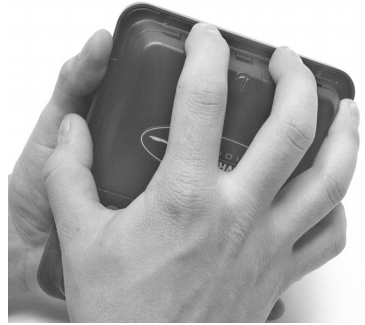
Loosen thumbscrew and remove AirMap battery cover.
